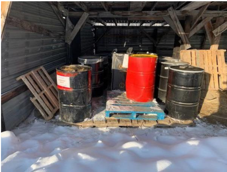
Photo 2: Sioux Lookout Camp and yard – One can labeled as antifreeze. Liquid hazardous waste requires a sufficient secondary containment. Each container should be labeled with contents as well as safe handling procedure.
