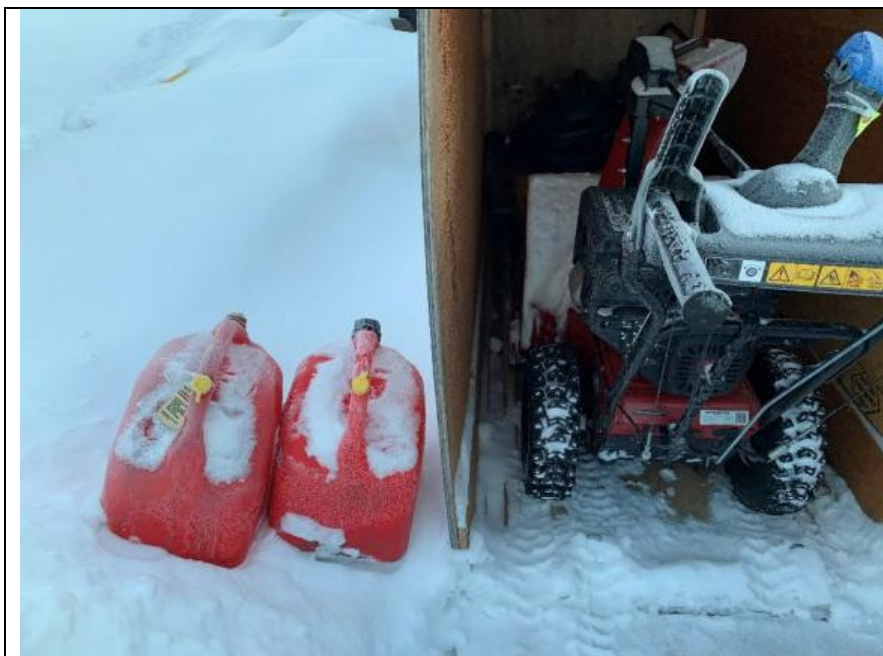
Jerricans stored without secondary containment. Missing WHMIS workplace label. Discussed with camp manager – Jan.
