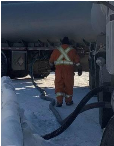
Fuel truck (third party) came by and started refueling. No spill tray was used, missing PPE (glasses, hardhat?).
