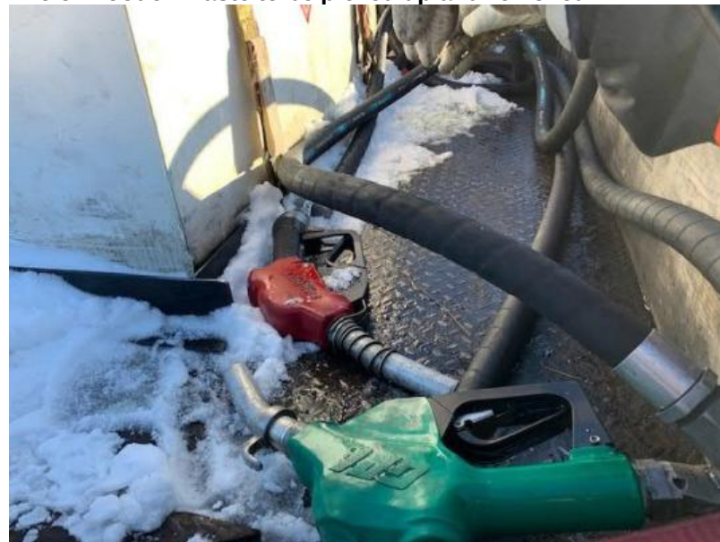
Hoses left in the back of the fuel truck are not stored properly and are leaking gas.
