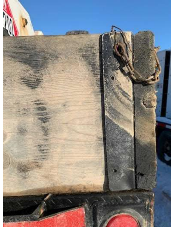
Staining from fuel on back of truck.
