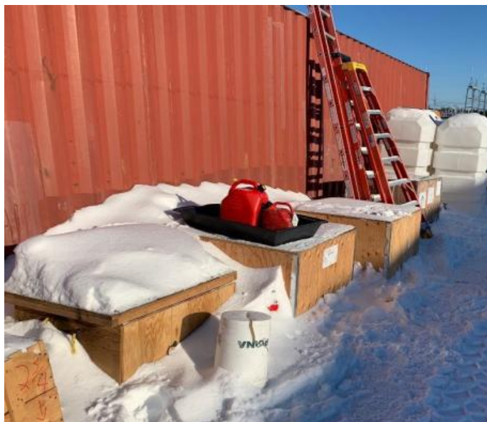
Jerrycans labeled (WHMIS) and stored on spill trays in Pipestone Camp.
