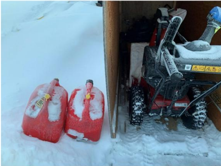
Photo 6: Sioux Lookout Camp and yard – Jerricans stored without secondary containment. Missing WHMIS workplace label. Discussed with camp manager – Jan.
