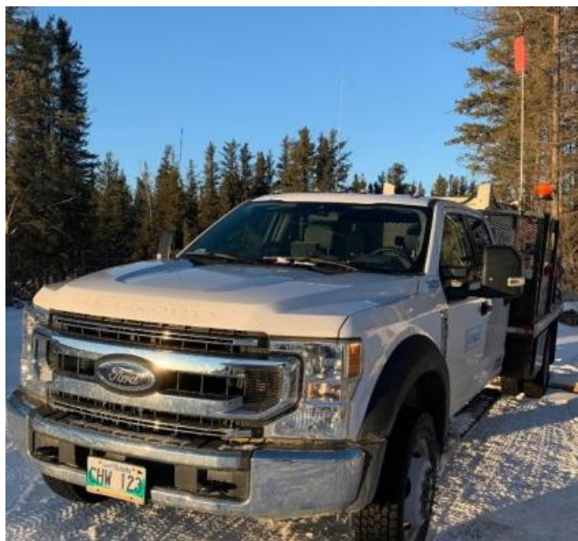
Photo 10: Pickle Lake Camp, Material Yard and Substation B – Mobile fuel truck parked at the material yard was missing the placard at the front of the vehicle.
